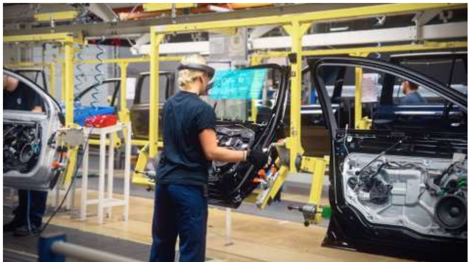
Using Hologlasses in Car Assembly [Erikson 2015]
